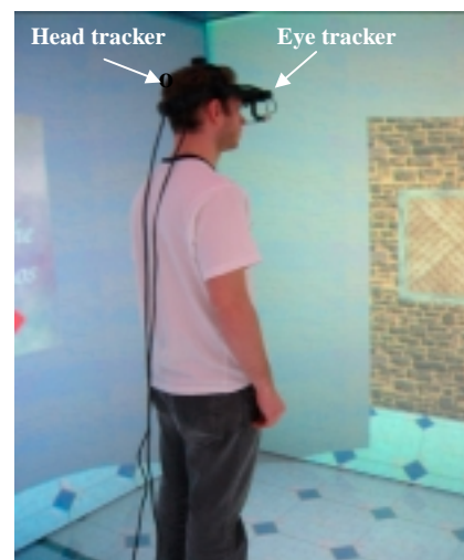
Figure 1: A subject wearing the head and eye tracker in IVY at York University.
