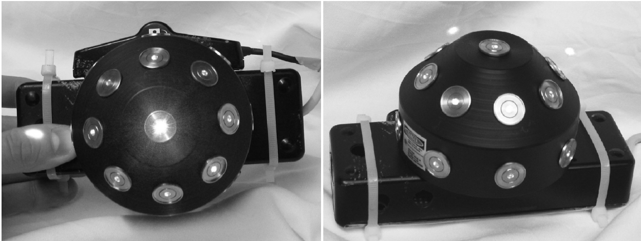
Figure 5. The Hedgehog hardware. A total of 17 laser diodes are arranged in a symmetrical hemispherical arrangement. As shown on the left, the IS-900 tracker is rigidly attached for experimental purposes.
