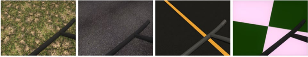
Figure 1. Examples of the terrains used in the low hover altitude estimation task. Each image was rendered in Autodesk MAYA™ 2016 at a simulated altitude of 5 ft or 1.5 m (from skid to ground). The terrains from left to right are the grass, stones, runway, and grid terrains, respectively. The same helicopter skid was visible in each image.
