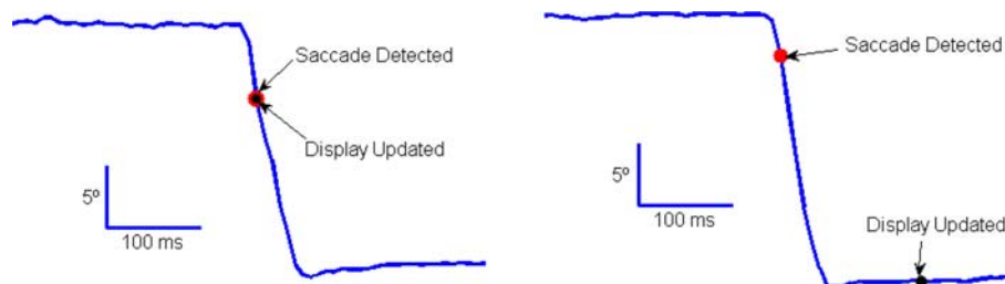
Fig. 2 Timing of saccade-contingent image displacements. Eye movement is shown as a function of time (proceeding to the right). The left-hand panel shows the timing of the scene change compared to the trigger for a trans-saccadic displacement. The change is programmed to occur as soon as the software detects the trigger condition (see text
