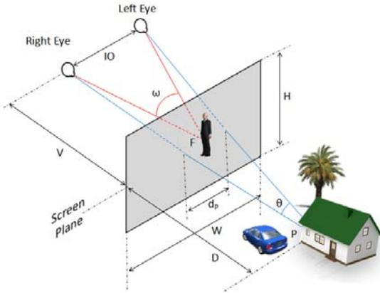
**Figure 1:** Here we illustrate the geometry of stereopsis with  $V$ : viewing distance;  $D$ : relative distance between an object  $P$  and the fixation point  $F$ ;  $IO$ : interocular distance;  $\omega$ : angle subtended by the eyes at the fixation point (screen plane);  $\theta$ : angle between eyes and the object;  $d_p$ : is the on-screen disparity of the point  $P$ .
