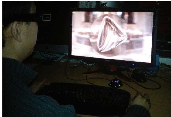
Fig. 2. Apparatus and experimental setup with subject. The subject viewed the image through shutter glasses and adjusted an overlaid gauge figure to match the surface normal direction by moving the mouse. The experiment was conducted in a dark room to control extraneous features and stray light.
