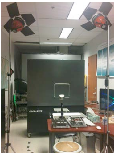
Figure 2. Experimental set-up showing the back-projection display, chin rest, and film lamps.
