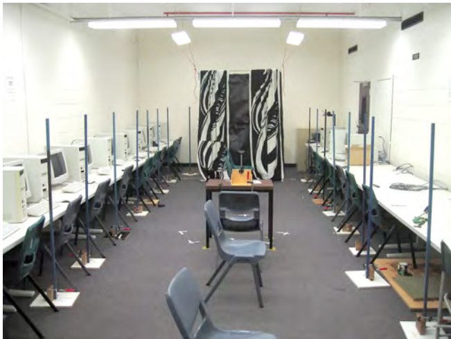
Figure 5 – Recent studies of stereoscopic depth constancy with targets at distances of between 4.5 and 200+ m were performed in large spaces, including a long laboratory (left, image from Allison et al., 2009) and a converted railway tunnel (right, image from Palmisano et al, 2010). Careful control of the target configuration ensured that only disparity cues were available to signal relative depth between the two LED targets. These targets can be seen through a slit in the black drape on the left hand side (barely visible in the photo due to their small size). The right hand side shows an elevated view with drapes removed so that more of the LED targets can be seen (only a single pair would be visible to the subject through a narrow slit). By controlling lighting we could provide rich distance cues to the layout of the surrounding environment while still restricting depth cues between the targets to disparity alone. When such cues were provided, considerable but imperfect stereoscopic depth constancy was achieved for target configurations starting at up to 40 m and with depth separations of up to 248m, well beyond the range of vergence as a distance cue.
