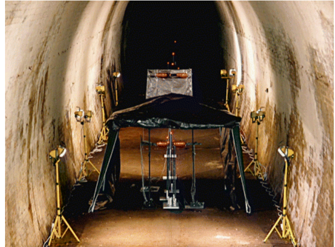
Figure 5 – Recent studies of stereoscopic depth constancy with targets at distances of between 4.5 and 200+ m were performed in large spaces, including a long laboratory (left, image from Allison et al., 2009) and a converted railway tunnel (right, image from Palmisano et al, 2010). Careful control of the target configuration ensured that only disparity cues were available to signal relative depth between the two LED targets. These targets can be seen through a slit in the black drape on the left hand side (barely visible in the photo due to their small size). The right hand side shows an elevated view with drapes removed so that more of the LED targets can be seen (only a single pair would be visible to the subject through a narrow slit). By controlling lighting we could provide rich distance cues to the layout of the surrounding environment while still restricting depth cues between the targets to disparity alone. When such cues were provided, considerable but imperfect stereoscopic depth constancy was achieved for target configurations starting at up to 40 m and with depth separations of up to 248m, well beyond the range of vergence as a distance cue.
