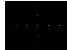
Calibration procedure: 5 points in both horizontal and vertical directions
