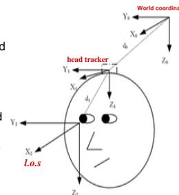
Measurement of eye and head position and orientation allows for estimation of the point of regard (gaze position). To measure the position of regard (POR) the intersection of the line of sight (l.o.s.) with the stimulus plane must be determined.
