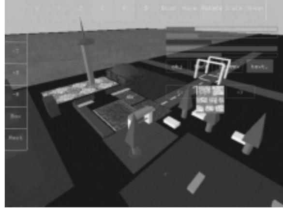
**Figure 4. The user interface: transparent buttons are overlaid over the rendered 3D environment. These buttons can be used to manipulate existing objects in the environment and to initiate the creation of new objects. The ‘brick’ pattern in the middle of the image is the currently selected texture for texturing existing surfaces.**
