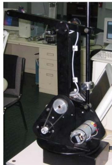
Figure 1. Photograph of the robot used for presenting haptic display to the subject.
