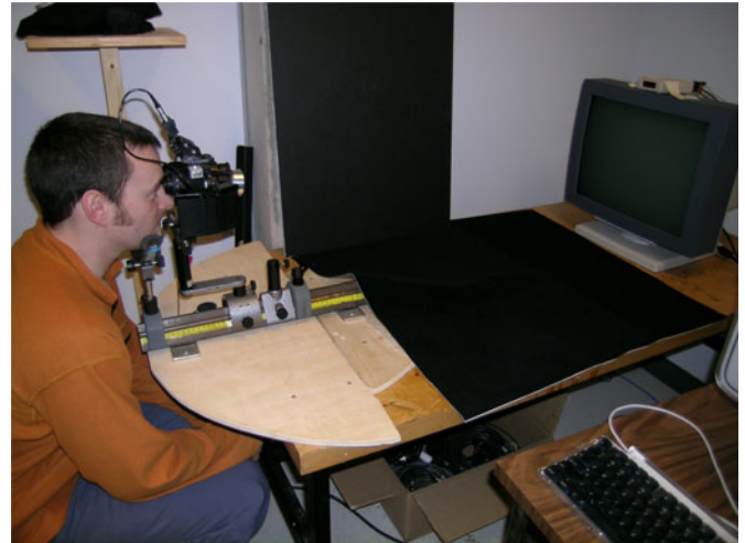
Fig. 1. Experimental setup. Observers viewed the display with natural vision or through night-vision devices at a distance of 120 cm with head stabilized with a chin rest. Black card and material used to block and baffle light has been removed for better visibility of the apparatus.
